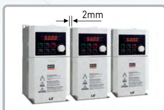
Side-by-side Installation (2mm between drives)
